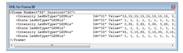
A note about animation optimization; When displaying the xml for an individual frame, both the Intensity and State values are listed for each LED controller. When the animation is saved to a .LWAX file, the Intensity values are optimized – they are only included for a frame if the values differ from the prior frame.
